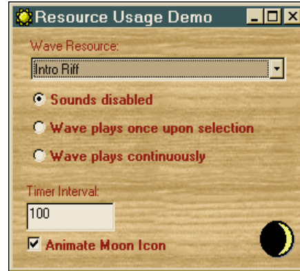
FIGURE 3 Multiple Effects Made Simpler with RES Files. This shows how you can use DrawIcon to place an icon over a painted background, preserving the icon's transparency. By rapidly calling DrawIcon with a series of icons, you can effectively duplicate the method
