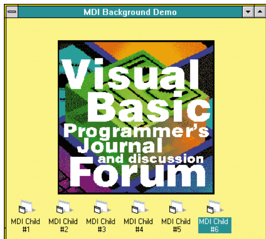
FIGURE 3 MDI Wallpaper. You can add your company's logo or other interesting bitmaps or patterns to an MDI background by intercepting WM_PAINT and WM_ERASEBKGD for the MDI client space.
